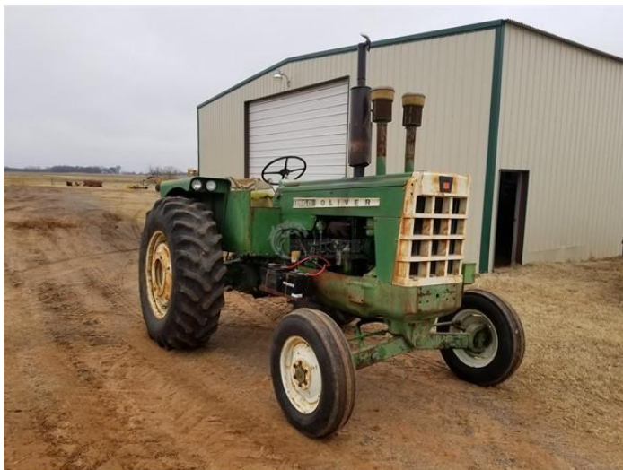
Oliver Standard 1950 (4-cil GM dieselmotor)
