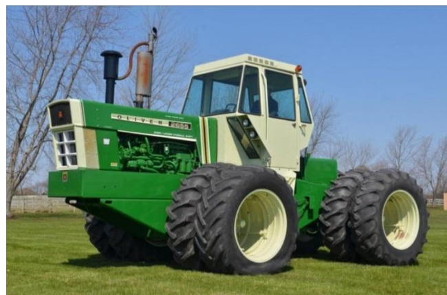
Oliver 2655 kniktractor (6-cil Minneapolis-Moline dieselmotor)
