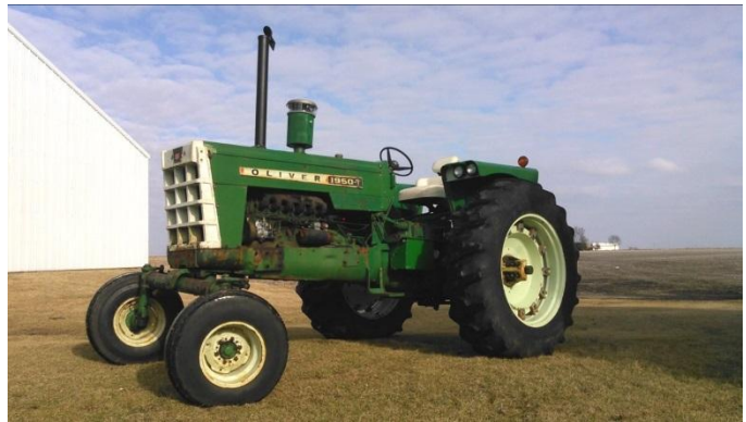
Oliver 1950-T wide front (6 cil Waukeseha Oliver diesel)
