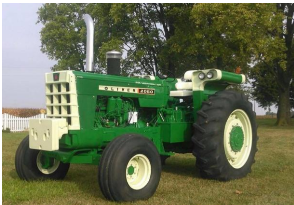
Oliver Wheatland 2050 (Hercules 6-cil dieselmotor)
