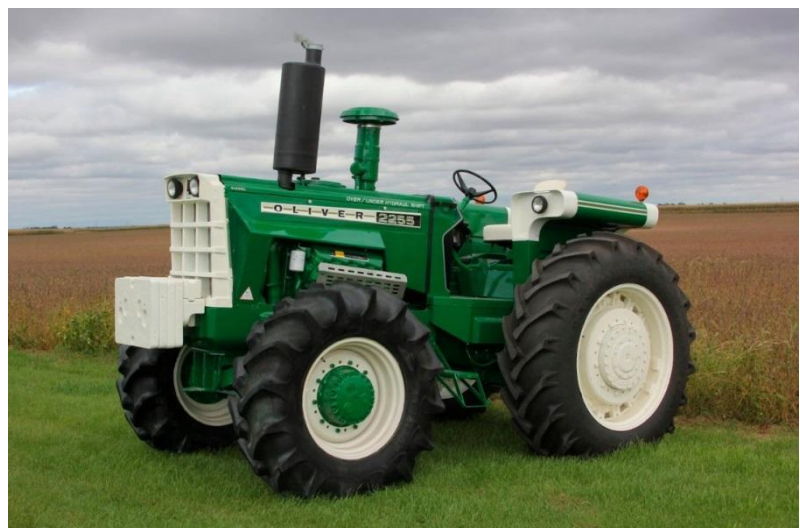
Oliver 2255 4WD (Caterpillar V-8 diesel)
