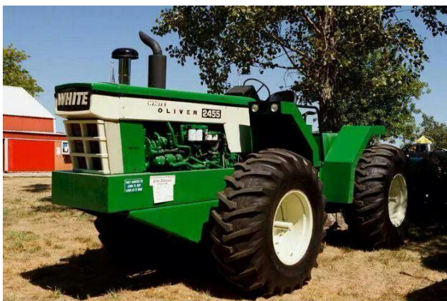
(Oliver 2455 kniktractor 6-cil Minneapolis-Moline dieselmotor)
